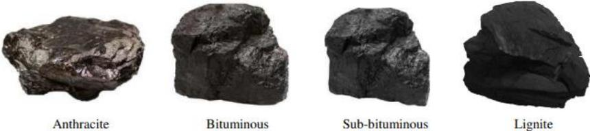
Type of coals which company distributes is Bituminous/Sub-Bituminous, as non-sized coal (0-50 mm), dust (0-5 mm and 0-10 mm) and nut (10-25 mm and 25-50 mm). Bituminous coal has Calorific value is high, moisture, ash and sulfur are low, so has the pollution environment much low, the industry is turning to coal as a replacement fuel.
